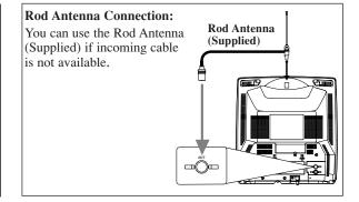
For your safety and to avoid damages to the unit, unplug the antenna cable from the ANT. jack before moving the unit.
